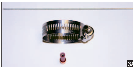
Figure 3: An O-ring clamp was used to determine the radius of curvature and the line perpendicular to the surface of the glenoid specimens (A). Note the hole drilled in the slots of the O-ring. The hole is just larger than the K-wires used for drilling. Another hole is drilled in the slot of the O-ring exactly opposite the superior hole. An extender guide (an electrical wire splicing device slightly larger than the 0.062-mm K-wire) was assembled to the O-ring clamp to keep the K-wire perpendicular to the clamp (B).
